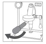
4) Remove the portafilter after extraction is finished by turning the portafilter handle from 7 o'clock to 6 o'clock position
