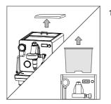
Open the top water reservoir cover and remove the water reservoir by pulling it upwards.
